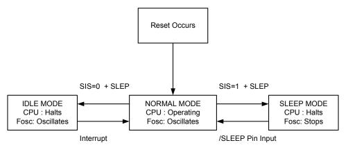
Fig 5. Operation Mode and Switching
